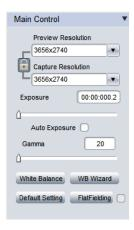
Note: The monochrome camera does not support the white balance function.
